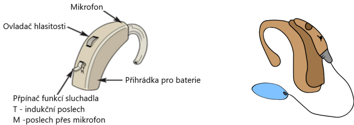
Fig. 2: Hearing aid and cochlear implant with T-switch
